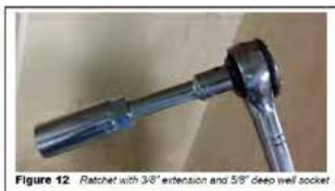
Figure 12 Ratchet with 3/8" extension and 5/8" deep well socket
