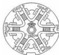
7-way trailer plug car end, rear view
